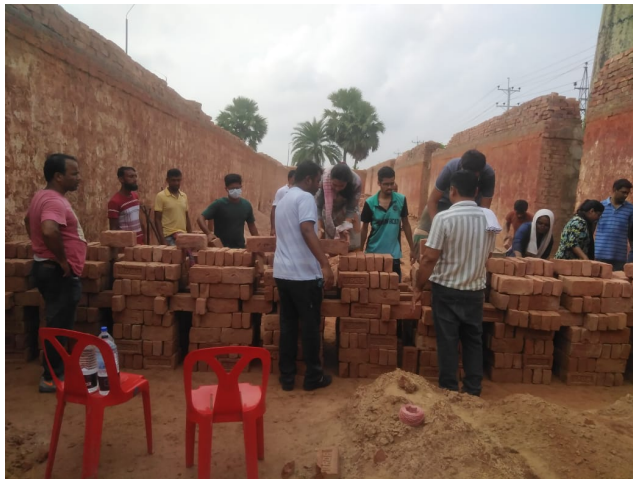
Figure 1: Double/Triple Zigzag brick stacking
