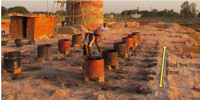
Figure 2: Continuous Coal Feeding
